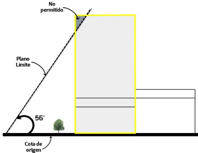
*Aplicación correcta de la Norma. Isométrico y alzado.*
